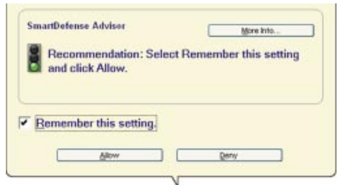
ZoneAlarm Internet Security Suite identifies programs by their MD5 “fingerprint” and provides advice on whether to allow or deny the program access to the Internet.
