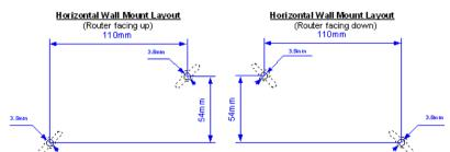
3. Mark two drill holes on the wall, in accordance with the following sketch:
