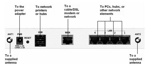
**Figure 6: Typical Connection Diagram**
